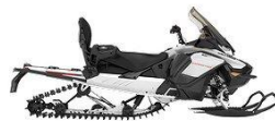
Skidoo Expedition Sport 900 ACE 95 hk 3923/ 406 /38,1 kam 4-takt motor 5 st Stor packlåda bak
